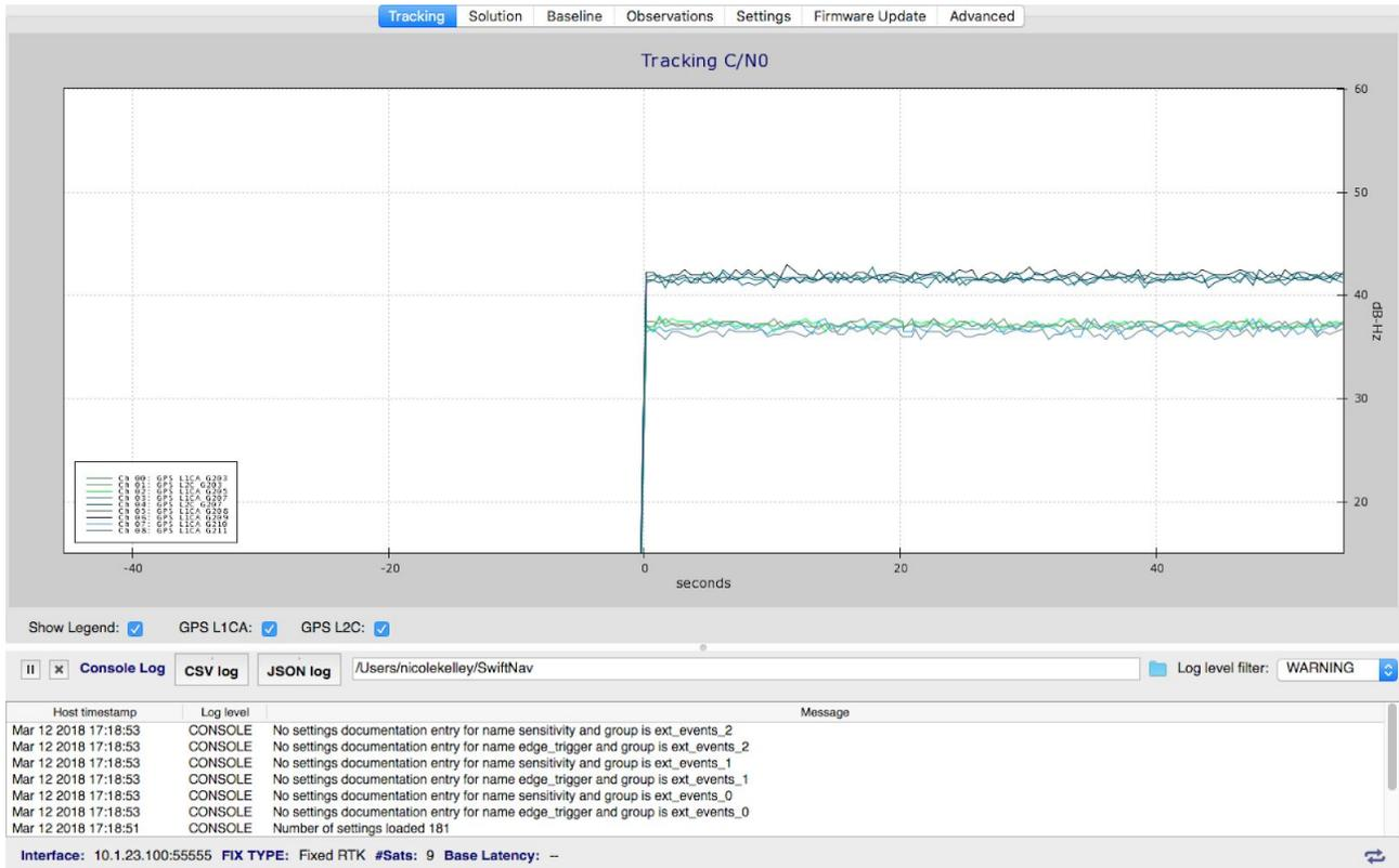
This tab shows the signals Piksi Multi is tracking. Each signal is represented by a colored line on the graph, and the line's position on the graph represents the strength of the satellite's signal over time.
