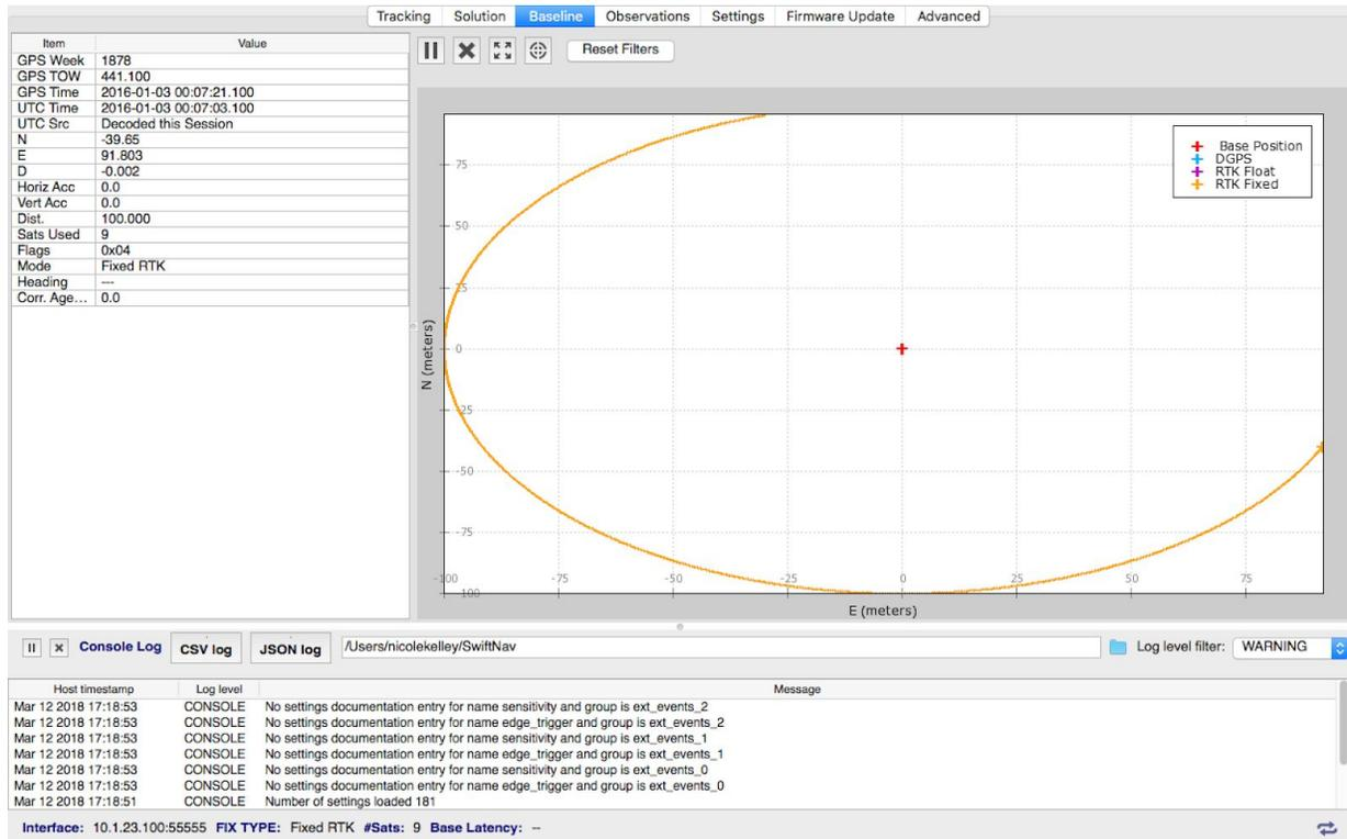
This tab shows Piksi Multi's RTK Baseline, a high-precision GPS position solution, with a relative position accuracy of few centimeters. This data visualization will show the base station as a red cross and the rover path in orange or blue.
