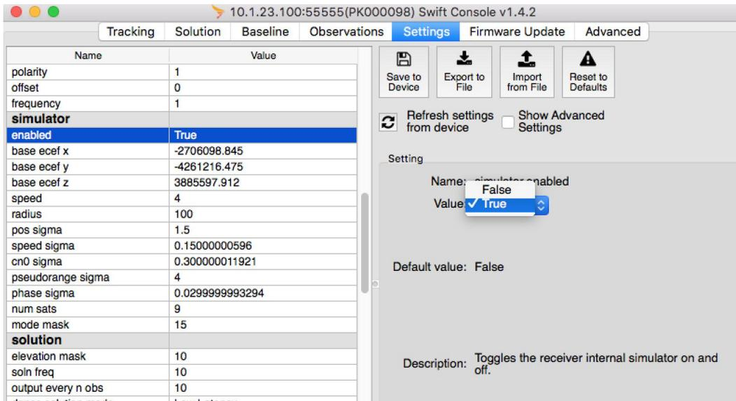
Your Piksi Multi will now be running in Simulation Mode. If you view the Tracking, Solution and Baseline tabs, you can now see the simulated output.
